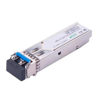
Small Form-Factor Pluggable (SFP) Fibre Optic Transceivers are compact transceivers used to interface networking devices to fibre or copper networking cables in telecom and data applications.
