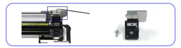
3 Disassemble and replace the Lever Block of left/right side with wrench as picture, as to fiber type.
