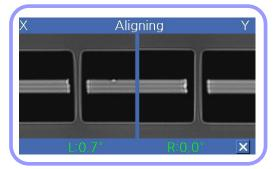
to be checked. If the measured cut angle is bigger than the preset limit value or any damage to the fiber is discovered, an error message appears on the screen and the splice process stops. If no error message appears on the screen, examine the condition of the cross sections with your eyes based on following figures. Any fiber that has similar condition to any of below figures has to be removed and a new fiber must be placed. These general defects can cause a wrong splice.
