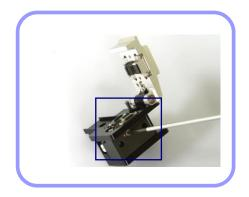
When the blade reaches required position, tighten the set-screw of the slider. Thoroughly and accurately set the height using a gauge because the height directly effects the cleave quality of fiber.
