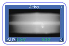
The splice loss value is measured after completing arc fusion and displayed on the screen. The loss value is affected by error elements. And, these elements also influence the estimation and computation of the value. The computation of the loss value is based on such clear measurement factors as MFD.
