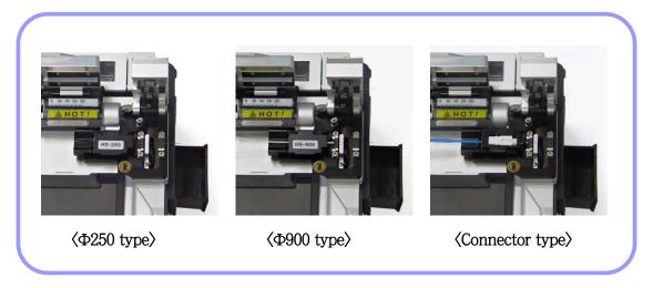
2 Press the cover to cleave the fiber.
