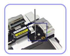
2 Open the cover and push the slider forward. When the slider is fixed, loosen the set screw a little bit (about 2 turns) with a hexagon wrench.
