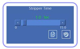
3 Select appropriate strip time by using ◀ or ▶ and confirm the adjustment by pressing ————.
