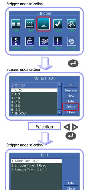
When is selected, temperature setting bar shows current set temperature.
