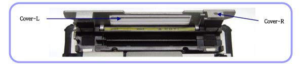
2 Disassemble and replace the Sleeve Heater Assembly with wrench as picture, as to fiber type.
