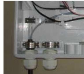
Connect small diameter cable with the splitter input cable by fusion splicing or mechanical splicing.
